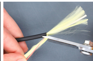
Step 4: At the interface of the 5mm jacket, cut off the ripcord and 50% of the Kevlar. **Note: If there are any excess fibers, cut off those as well.
