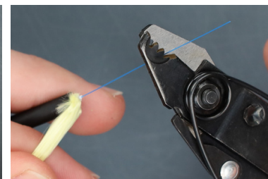
Step 7: Strip off the 250 μm coating back to the added mark—stripping off the mark in the process.
