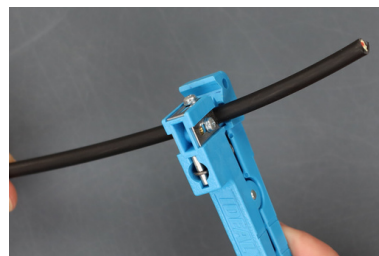
Step 3: Strip the outer jacket at the marked spot
